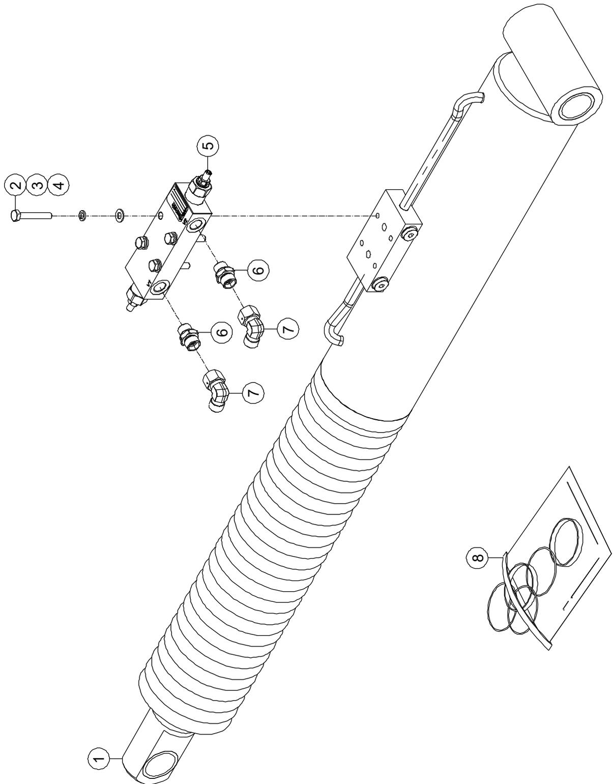
**5-6 JIB Leveling Cylinder Assembly (BT34BERT)**
