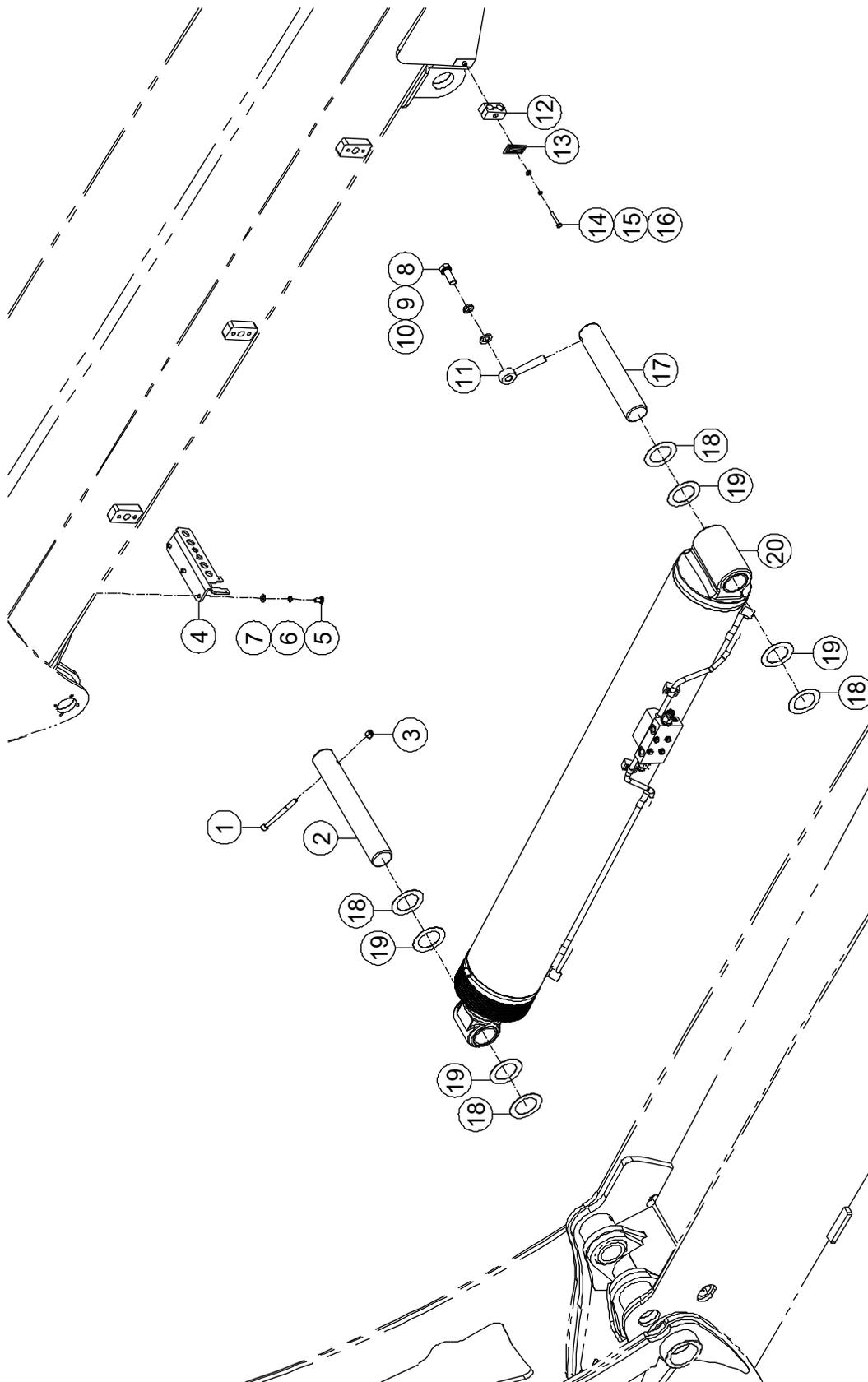
**3-4 Lifting Cylinder Assembly and Boom Installations**
