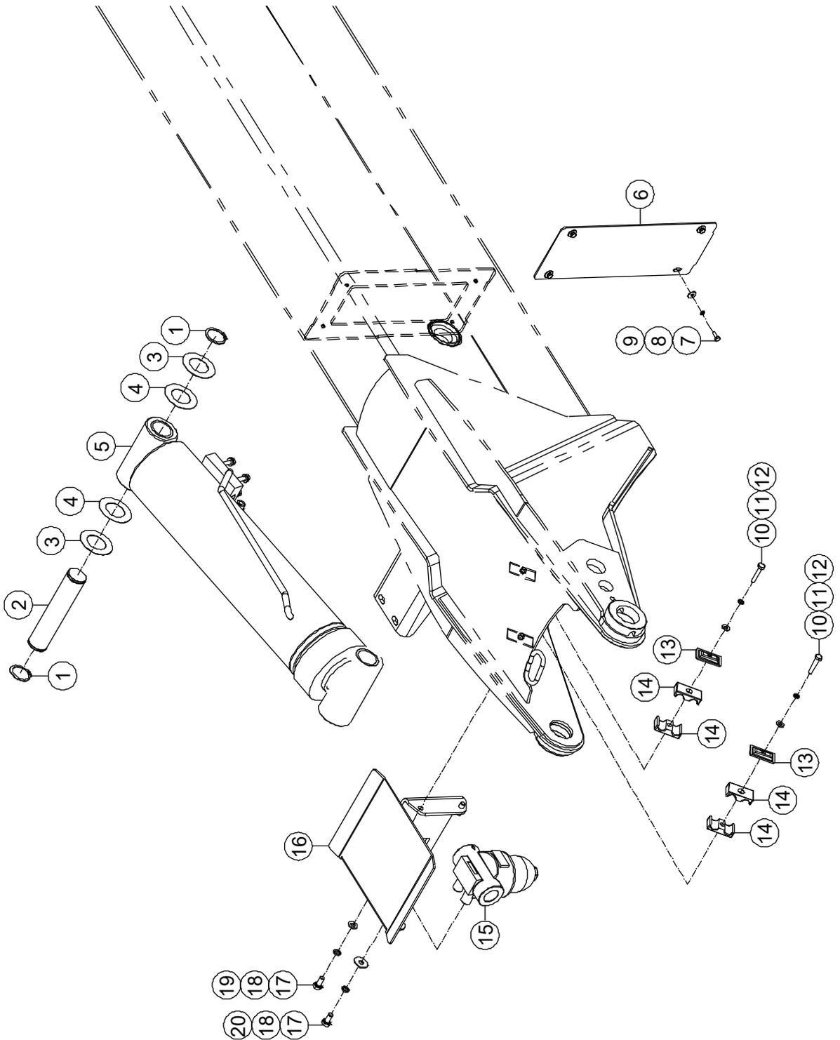
**3-17 JIB Leveling Cylinder Assembly Installations (BT34ERT)**
