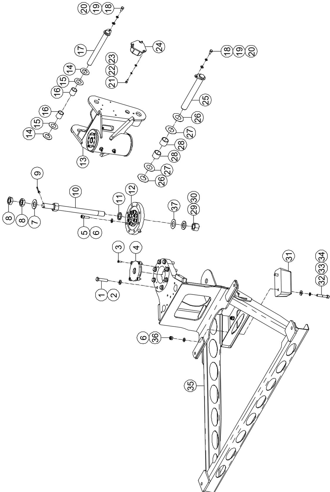
**3-23 Rotate Cylinder Assembly Installations**
