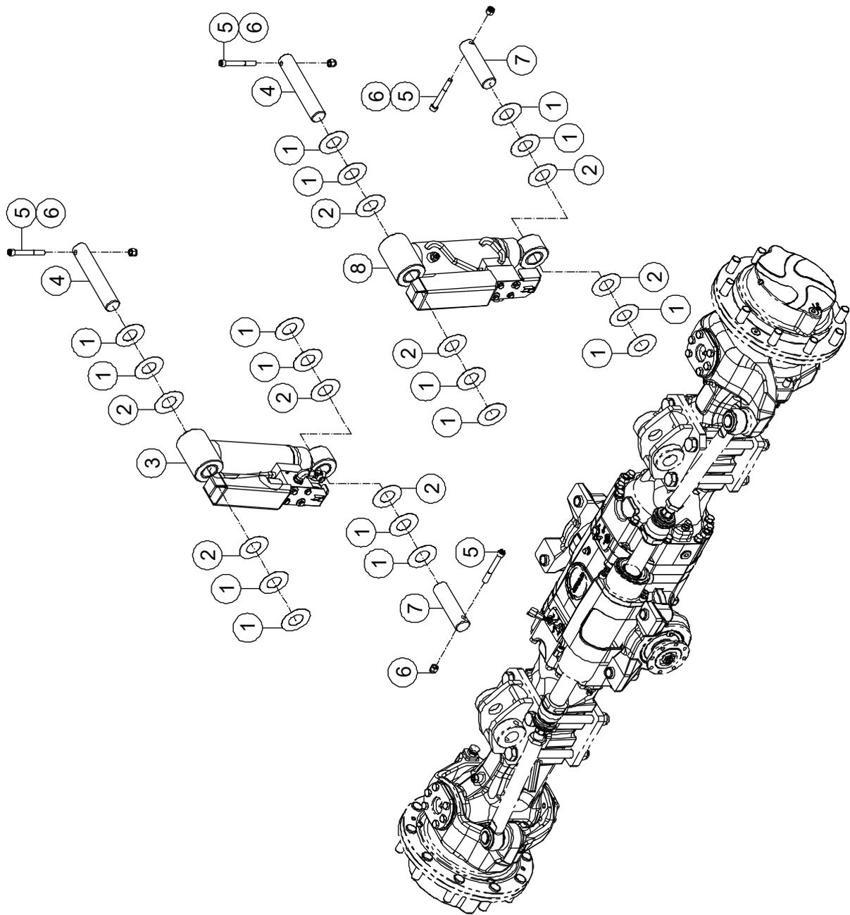
**1-3 Axle Lockout Cylinder Installations**
